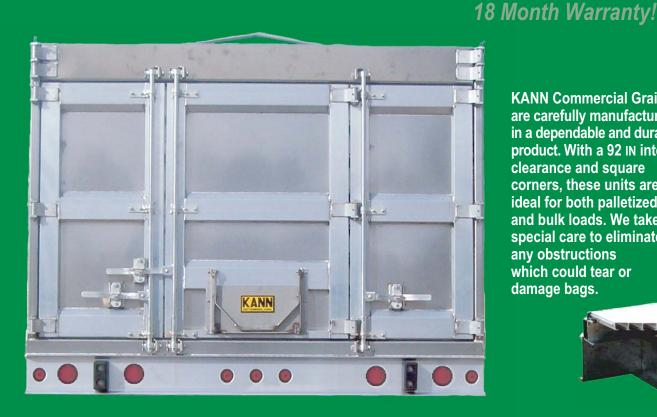
**KANN Commercial Grain Bodies** are carefully manufactured resulting in a dependable and durable product. With a 92 IN interior clearance and square corners, these units are ideal for both palletized and bulk loads. We take special care to eliminate any obstructions which could tear or damage bags.
