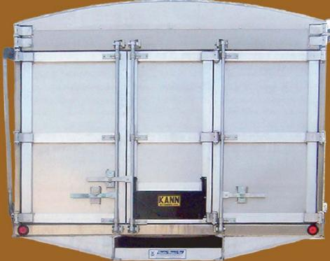
KANN Farming Aluminum Grain Bodies are carefully manufactured resulting in a dependable and durable product. With a 92 IN interior clearance and square corners, these units are ideal for both palletized and bulk loads. We take special care to eliminate any obstructions which could tear or damage bags.
