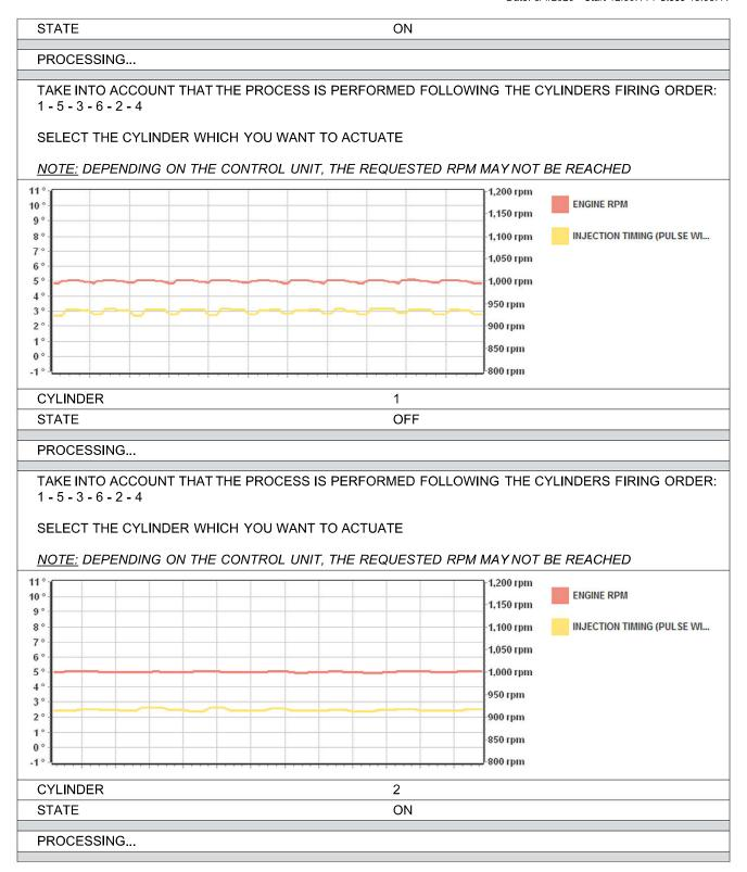
TAKE INTO ACCOUNT THAT THE PROCESS IS PERFORMED FOLLOWING THE CYLINDERS FIRING ORDER: 1 - 5 - 3 - 6 - 2 - 4
