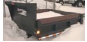
8' Heil Dump Body, Electric over Hyd Pump & Hoist, w/Subframe $950.00 SP 24180100
