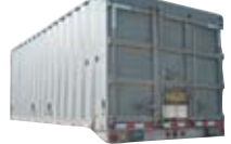
17' Kann Alum. Body, 2 Cyl Scissors Hoist, 94" Wide, 72" sides $7000.00 SP 24186674
