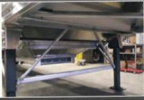
Standard on all Platinum Series aluminum subframe grain hoppers are hot dipped galvanized steel supports which connect the subframe to the crossmembers. In combination with the aluminum subframe, this offers a more durable and corrosion resistant solution.
